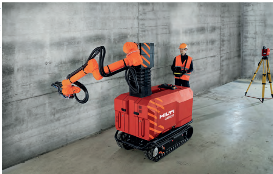
ABOVE: Hilti Jaibot robotic drill.
